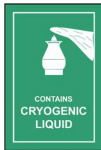
Figure 6. Handling label for cryogenic liquids; for transport by air, where cryogenic liquids (deeply refrigerated liquefied gases) are used (see section on Refrigerants), this label shall be affixed to insulated vessels or flasks used as outer packaging in addition to the labels or markings shown in Figures 3, 5 and 10, as appropriate
