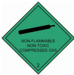
Figure 5. Hazard label for liquid nitrogen; substances packed using liquid nitrogen (see section on Refrigerants) shall bear this label in addition to the primary risk label (e.g. the label shown in Figure 3 for Category A infectious substances, the marking shown in Figure 10 for Category B infectious substances)
