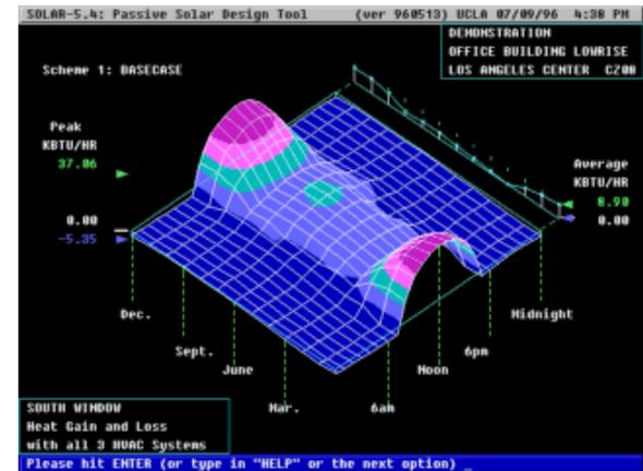
•**Energy 10 (\$50)** Design tool for smaller residential or commercial buildings that are less than 10,000 ft<sup>2</sup> floor area, or buildings which can be treated as one or two-zone increments. Performs yearly whole-building energy analysis, including dynamic thermal and daylighting calculations. Passive Solar Industries Council.
