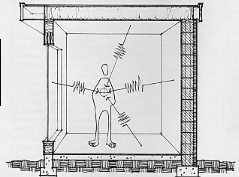
Mean radiant temperature (MRT) is the weighted average of the various radiant surfaces within a space.
