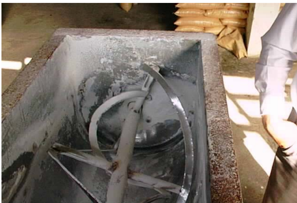
Figure 4: Two Ton Capacity Batch Ribbon Mixer, at Refineria Dominicana de Sal
