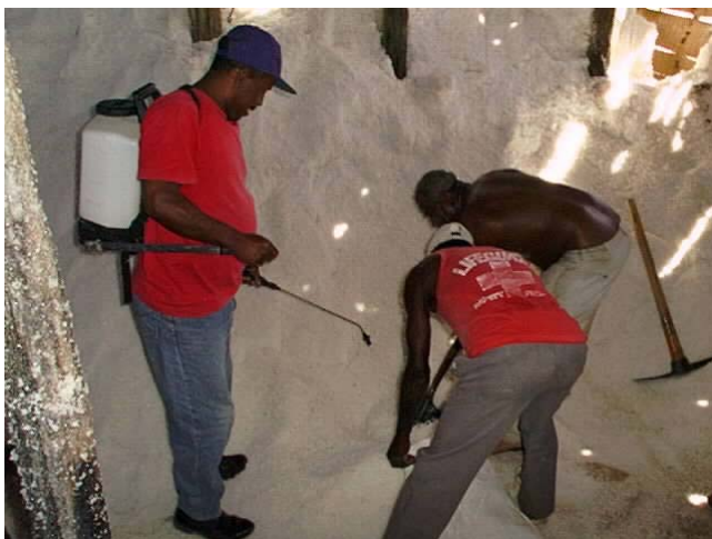
Figure 15: Iodization of Crude Salt by DISSAL personnel
