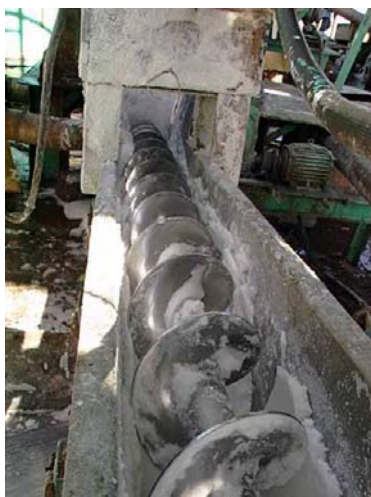
Figure 9: Discharge from Centrifuge to Screw Conveyor.
