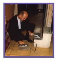
*Figure 12:* Peru, 1966—Regional advisor checking for alpha contamination in radium-loading room.
