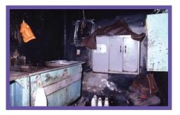
*Figure 11:* Poorly maintained darkroom; note broken "safety light" replaced by a paper bag covering a common light bulb.
