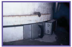
*Figure 39: D*evice showing how each drawer could be moved in to place to give access to the radium needles.
