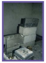
*Figure 27:* Improvised shield to test whether sources were leaking.
