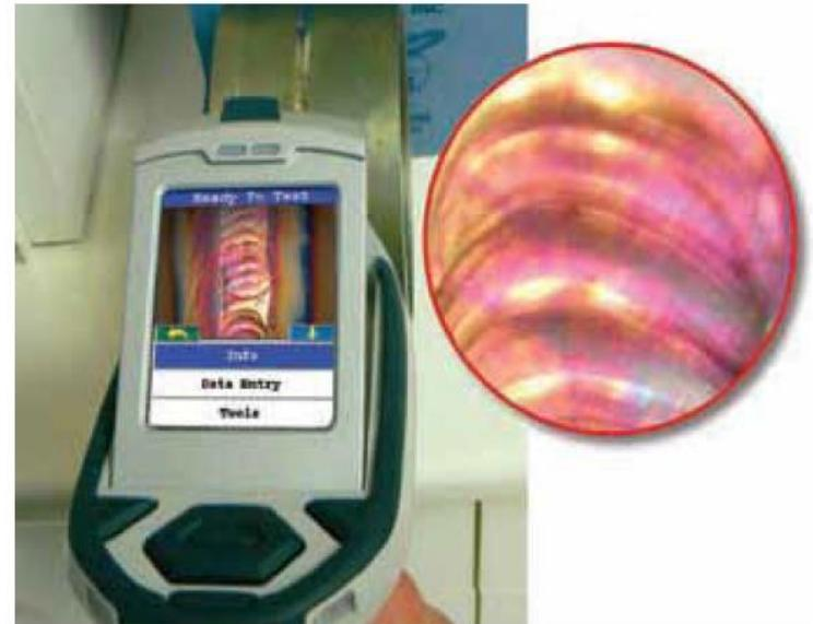
CCD camera and small-spot feature isolates and stores small sample area measurements.
