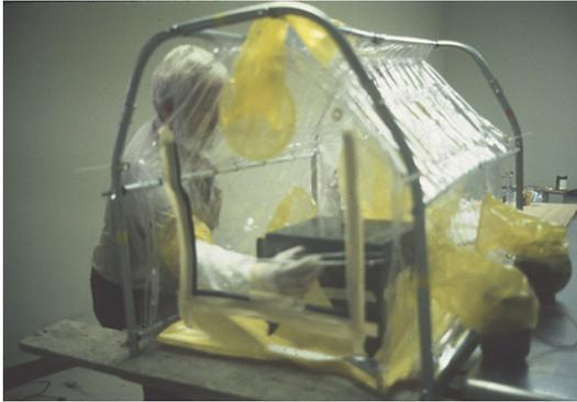
*Figure 22:* Disposable glove box used to remove radium sources from Instituto del Cibao, Santiago de los Caballeros, Dominican Republic, 1991.
