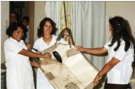
Figure 10: Honduras, 1975— Technologists with defective protective apron.
