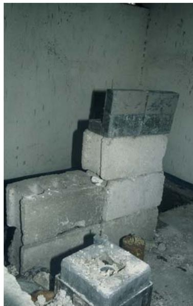
Figure 27: Improvised shield to test whether sources were leaking.
