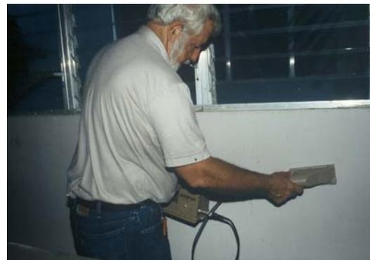
*Figure 25 (above):* Checking for residual radioactive contamination.
