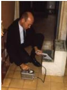
Figure 12: Peru, 1966—Regional advisor checking for alpha contamination in radium-loading room.
