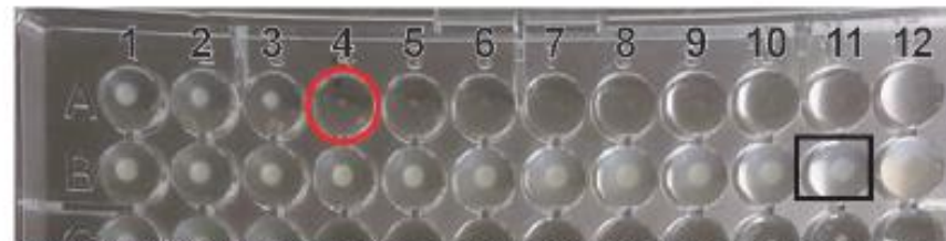
Figure 12. Cefiderocol Test With a Trailing End Point. The cefiderocol concentrations in wells A1 to A12 are 0.03 to 64 \mu\text{g/mL} . Row A shows the cefiderocol MIC at 0.25 \mu\text{g/mL} in well A4 (red circle). The growth control well is B11 (black box).
